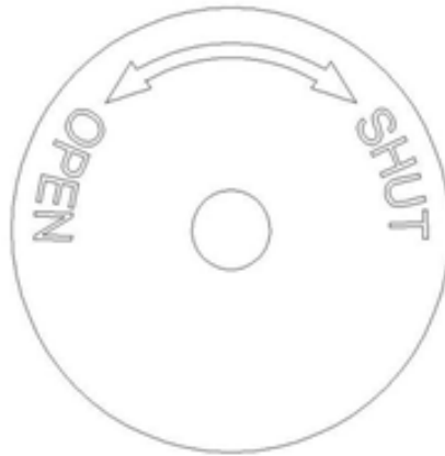
Figure 2: Hand wheel indicator for opening and closing signs
